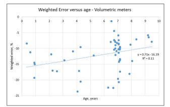
Figure 7. Weighted error versus age – volumetric meters
