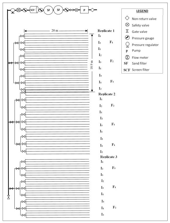
Figure 1. Schematic sketch of micro-irrigation system components and treatments
