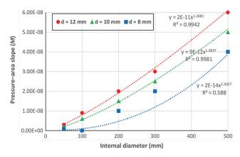
Figure 6. Variation in elbow internal diameter against pressure-area slope
