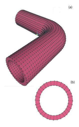
Figure 1. Geometry of the elbow model: (a) 3D model; (b) Crosssection of the model
