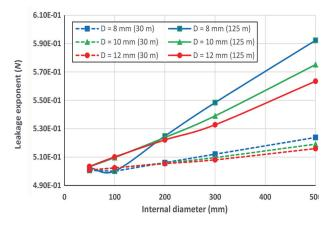
Figure 12. Leakage exponent versus elbow internal diameter for various pressures
