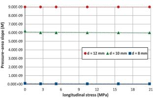
Figure 8. Variation in longitudinal stress against pressure-area slope
