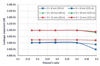
Figure 13. Leakage exponent versus Poisson's ratio for various pressures
