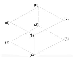
Figure 2. Solid element joint connectivity
