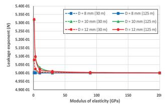
Figure 11. Leakage exponent versus elastic modulus for various pressures
