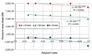
Figure 7. Variation in Poisson's ratio against pressure-area slope
