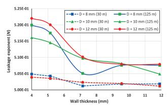
Figure 15. Leakage exponent versus elbow wall thickness for various pressures
