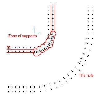
Figure 3. Boundary conditions (supports) of the elbow
